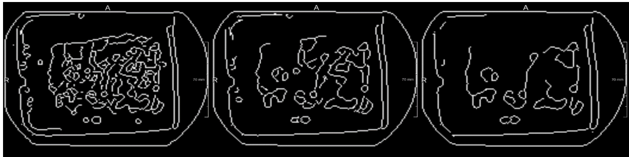
Figure 4.23: Results of the Canny edge detector on another dataset preprocessed by unsharp masking. Sigma value used are 3, 5, and 7, with low threshold of 0.02, 0.03, and 0.04.
