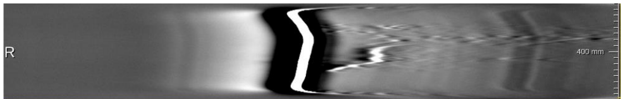
Figure 4.31: Time-domain side view of the same dataset. Tumor region beneath the paraffin covering and block surface shows a strong reflection response and is easily identifiable.
