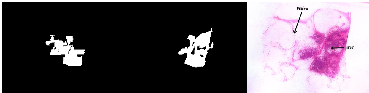
Figure 4.27: Region growing using our C++ program from a single seed point. The left image is generated by comparing adjacent time sequences. The middle image is generated by comparing with the initial seed point only. The right image is the histopathology image for comparison.
